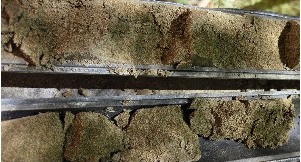
Plate 5 – Pre-Olympia, Non-glacial Coarse Grained: Very dense fine SAND with silt (Qponc) | PG-1-25, S-9 @ 25-26½ feet.
